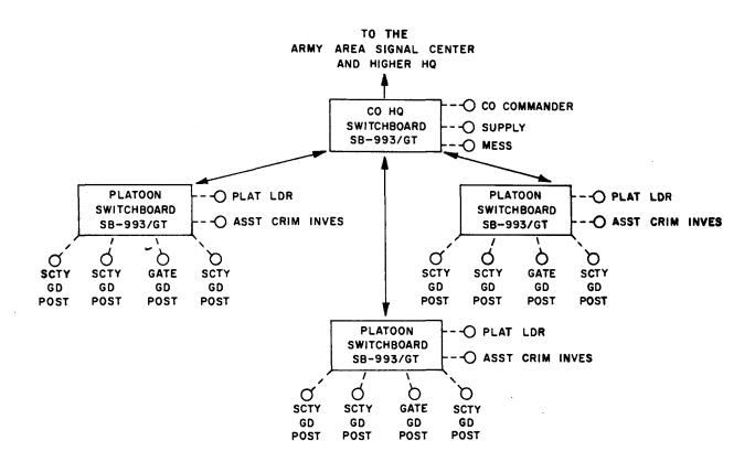
Figure 56. Wire communications diagram, military police physical security company.
